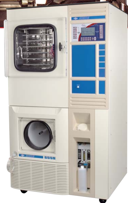
Genesis 35 EL with bulk shelves and automated Wizard 2.0 Control System
